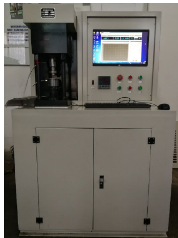
Figure 7 Photograph of the ring-on-disk tribometer
