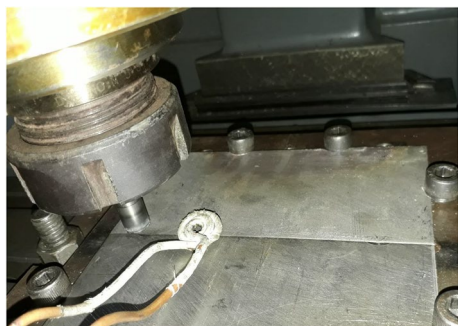
Figure 33 Induction assisted friction stir welding setup [237]
